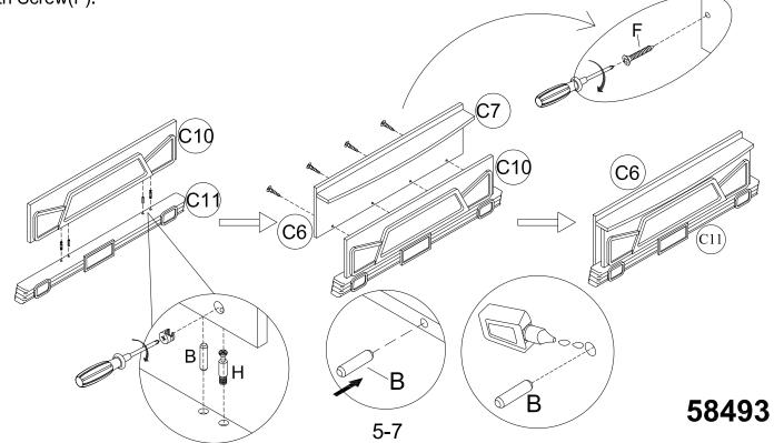
STEP 5: Insert the Dowel(B)to the Left siderail(C3).use Hex Key(G)to tighten the Headboard Inside Panel (C6)and Headboard Front Panel(C10) and Headboard Top Panel(C4)and Headboard Top Apron(C5) and Footboard (C13)to the Left
